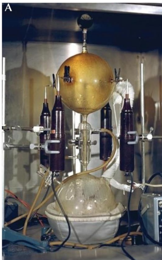
FIGURE 4.6. The apparatus used in the Miller–Urey experiments. (A) Recreation of the original apparatus. (B) Diagram of the apparatus.
