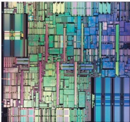
**FIGURE 24.26.** The placement of components on a computer chip is often designed by a **genetic algorithm**, which uses natural selection to search for the optimal solution. This microprocessor contains 15 million transistors.
